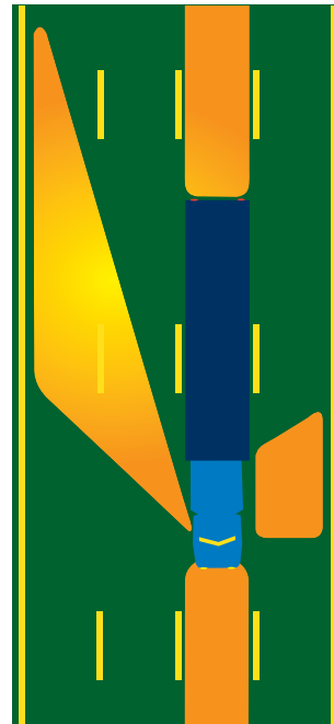
Represents danger areas around trucks where crashes are more likely to occur.
