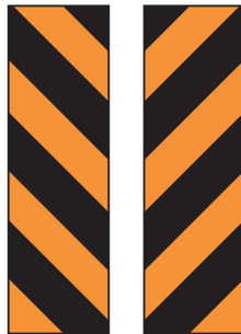
Hazard to left Hazard to right
